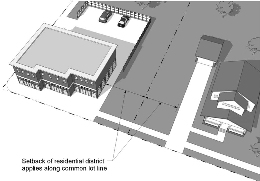
Figure 3.7.5-A: Transition of Side Yard Setbacks
